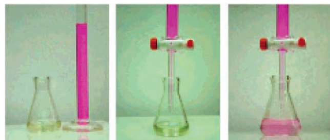
Figure 3. Use of the scavenger 10 in a Diels–Alder titration experiment, scavenging an excess of 11 after a Diels–Alder reaction with DMAD: left, 0.005 M solution in CH 2 Cl 2 ; middle, before equivalence point; right, at equivalence point.
